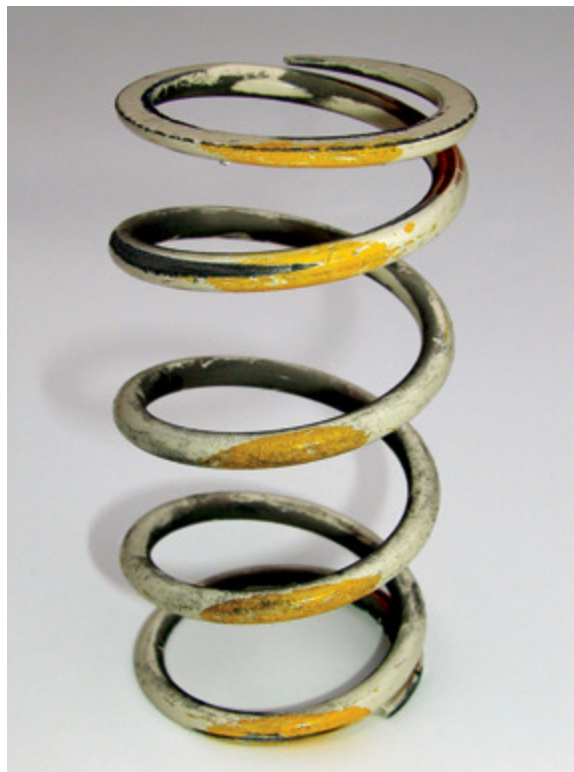
Drive clutch springs should be inspected for deformation and measured for proper free length (sagging). They should be replaced each year or every 2000 miles for consistent performance.
